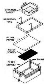
Figure 1.3: Assemble filter
